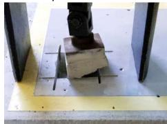
4EVER CONCRETE FLOOR Paint's adhesion was so strong that it cracked the concrete.
