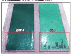
4EVER CONCRETE FLOOR Paint was painted over an oil-soaked substrate
