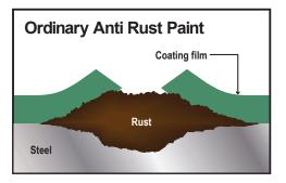
Coating film is broken by rust. Rust begins to spread gradually.
