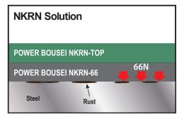
[POWER BOUSEI NKRN-66] strongly presses rust with 66N pressure. In addition, strong and highly flexible [POWER BOUSEI NKRN-TOP] prevents rust for a long time.
